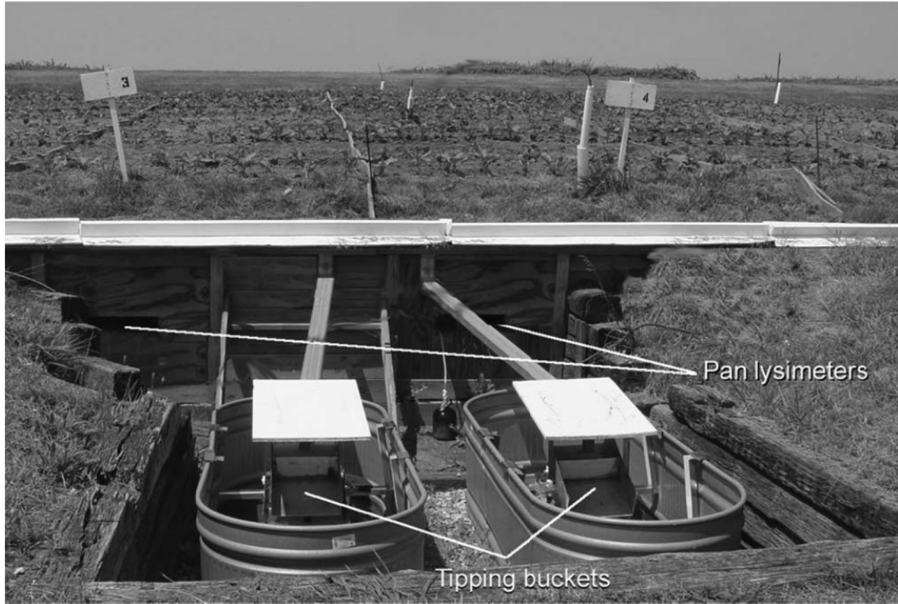
Fig. 2. Design of tipping bucket apparatus ( n = 18 ) installed down the farm slope at Kentucky State University research farm (Franklin County, KY). One tipping bucket apparatus for each of the 18 experimental plots for measuring and collecting runoff water samples.
